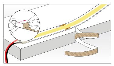
**3** Remove the adhesive tape, position the COB strips carefully, ensuring they are straight, and press firmly. Avoid removing and reapplying the strip (see Figure 1 on page 2).
