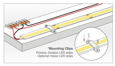
WAGO connectors enable quick wiring of LEDs in series. Use mounting clips and screws that match the width of the strip to support the COB strip light.
