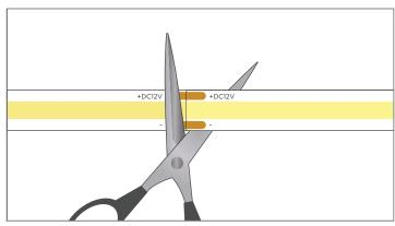
**2** Cut the strip to the required length by following the cutting mark, ensuring that you prevent damage to the light.
