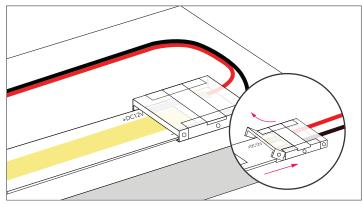
4 Our \*COB Strip Connector enables quick, solder-free joining of wires or COB strips. Various connector types are available to suit specific applications (see Figure 2, page 2).
