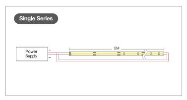
Do not exceed the maximum length of COB strips per series (refer to each item's spec sheet). We recommend wiring both ends of COB strips to the power supply.
