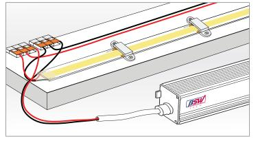
**6** Wire both ends of COB strips to the power supply. For multiple series, connect them in parallel to avoid voltage drop and ensure brightness.(refer to Figure 3 on page 2)
