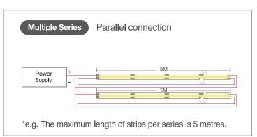
If you require **multiple strips**, they must be wired in parallel as a safe electrical operation mode. **Serial connection is not recommended**, as unbalanced voltage drops can lead to hazardous overload, potentially damaging the COB strips and causing uneven brightness.
